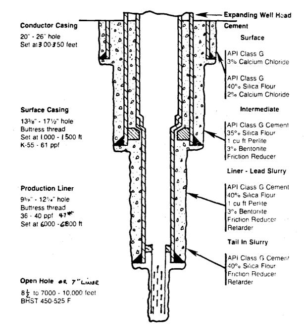
Note - Liner top sometimes squeezed tie back string usually 10%. All slurries mixed with 0% free water. Preflushes used on all strings. GEOTHERMAL WELL PROGRAM
