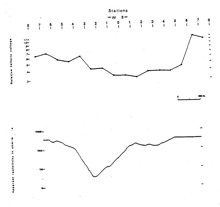
Fig. 3. E-field ratio telluric data for traverse 1 (top) and AEM apparent resistivity for flight line 407. Analogue equipment recorded the EM data at approximately 3600 Hz.
