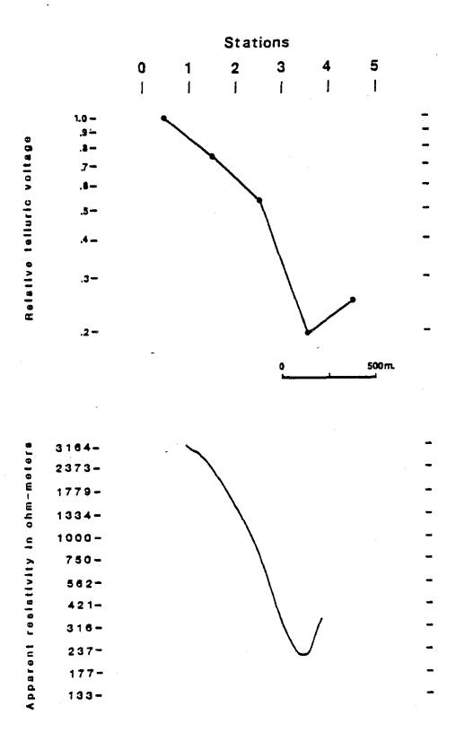
Fig. 6. E-field ratio telluric data for traverse 3 (top) and AEM apparent resistivity from contours of flight line 410. Analogue equipment recorded the EM data at approximately 3600 Hz.
