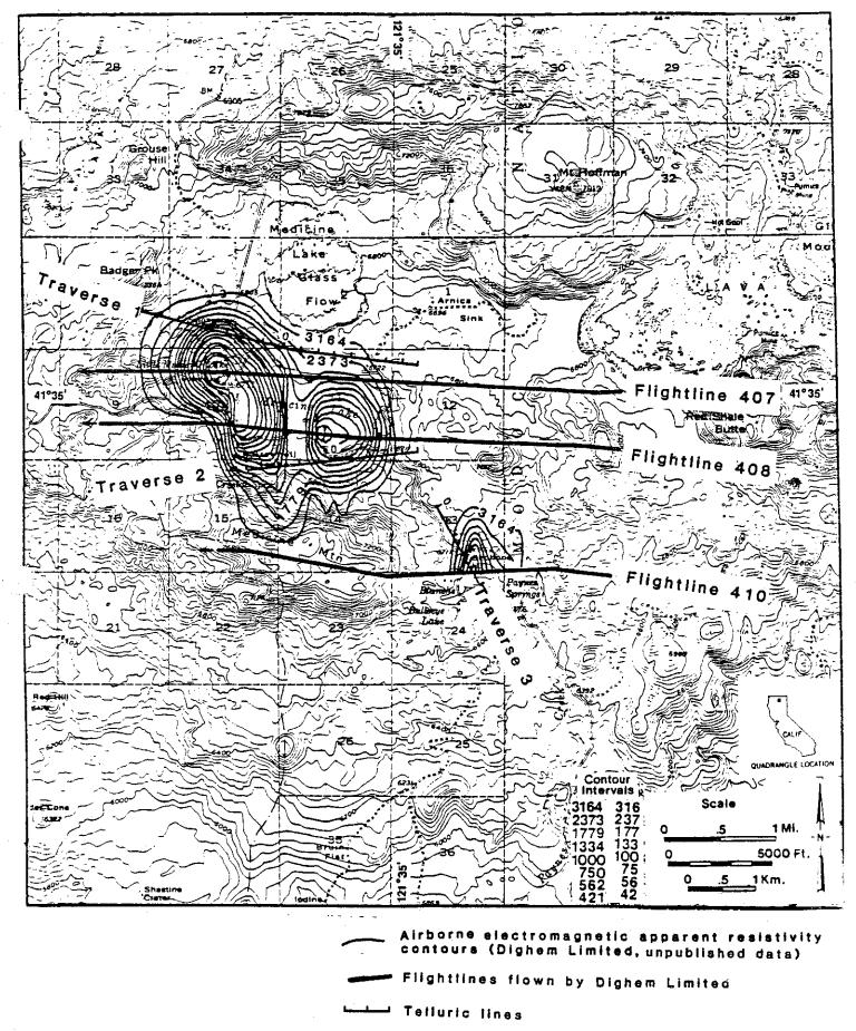
Fig. 4. Location map of telluric traverses and AEM apparent resistivity anomalies.
