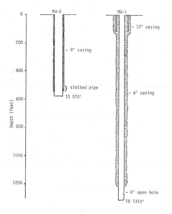
Figure 2 Well Construction
