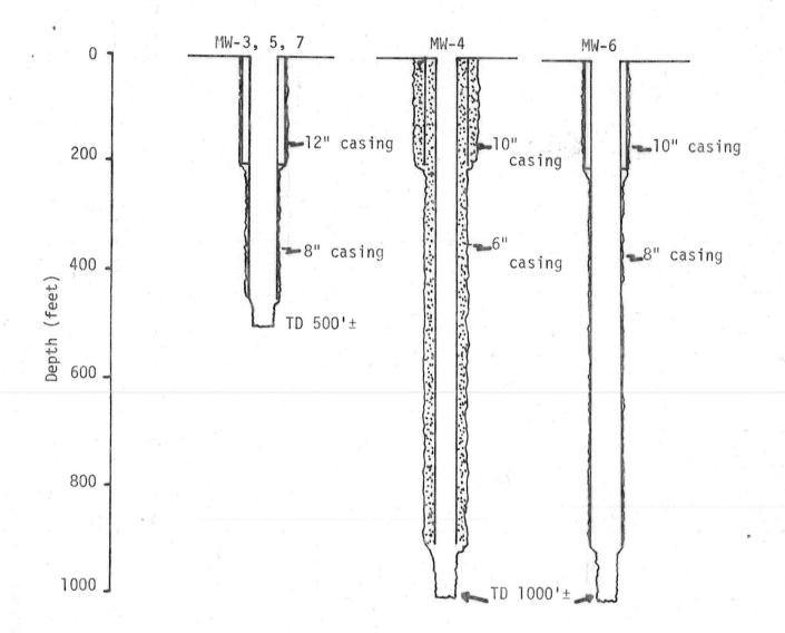
Figure 3 Well Construction
