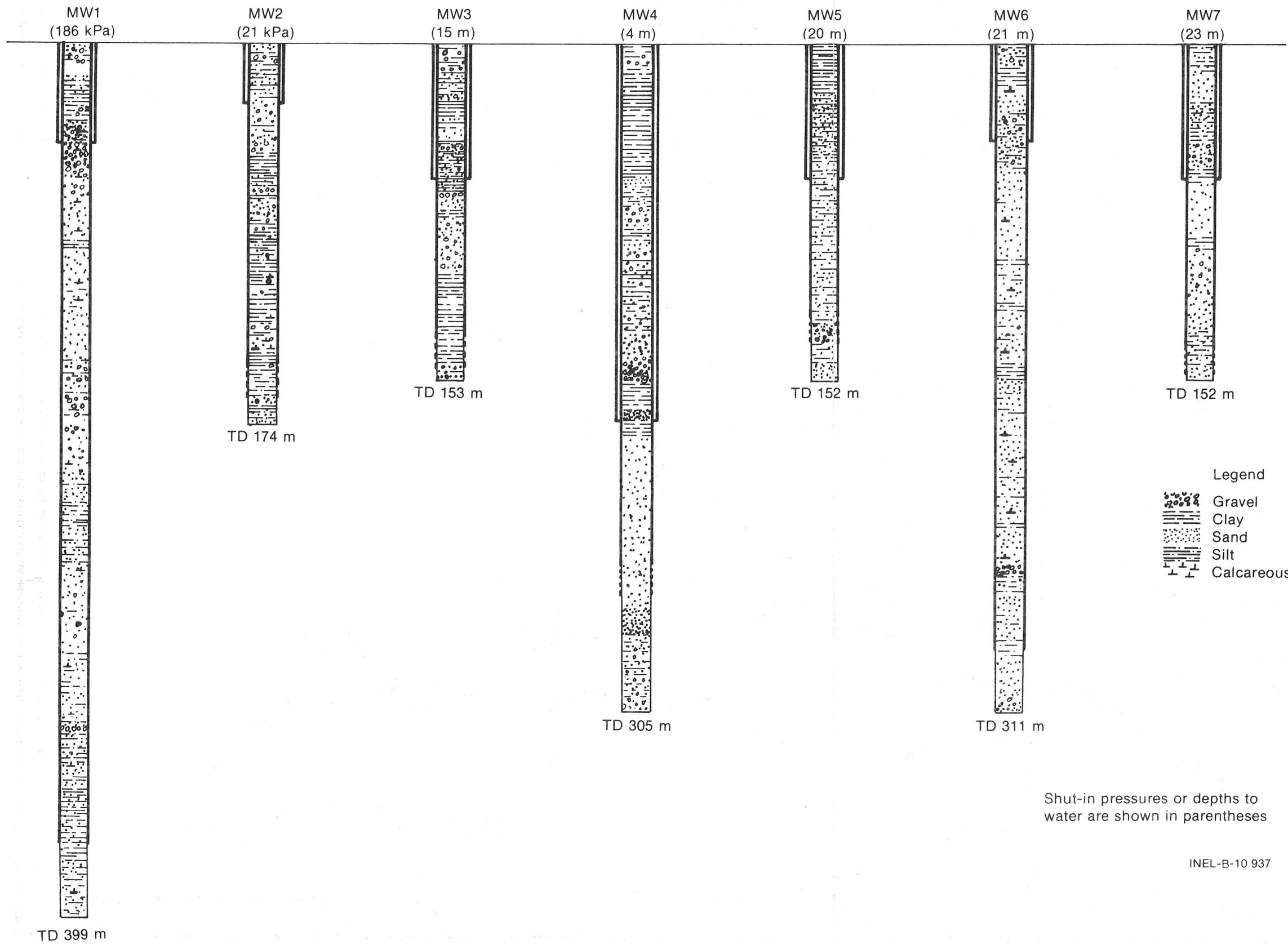
Fig. 10 Construction and lithology of monitor wells.
