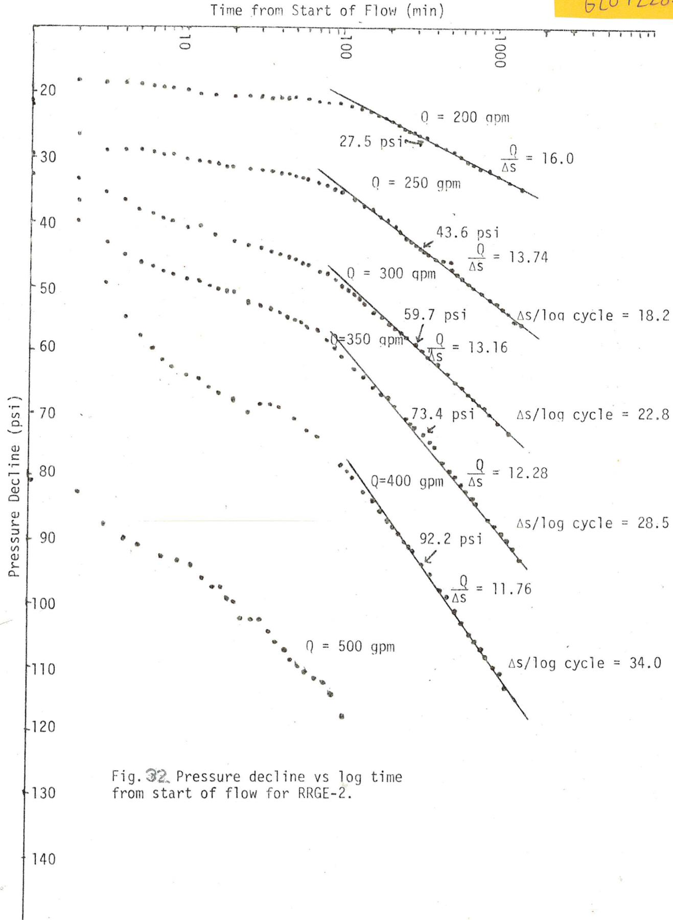
Fig. 32. Pressure decline vs log time
